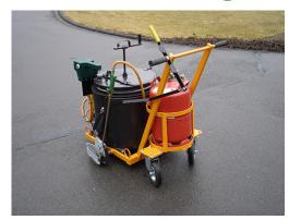
Melting and sealing device for melting and filling bituminous joint sealing material
