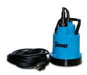
Powerful, portable all-metal pump that removes water up to a height of approx. 2 mm above the floor surface via the protected floor inlet. The pump already starts working at a water level of only 5 mm! Hose connector for ½", ¾" and 1" hose.
