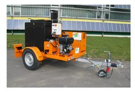
Equipment for melting and processing thermoplastic road marking materials
