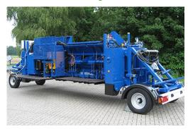
For automatically installation of mastic asphalt for road building with automatic grit
