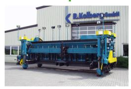
For automatically installation of mastic asphalt during road building with automatic grit
