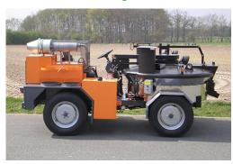
Special equipment for the transport of mastic asphalt at the construction site
