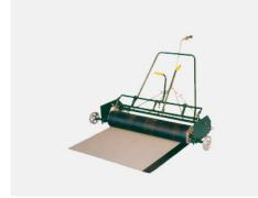
Offering many advantages through advantages through advanced technology. There is a short controlled flame running the width of the roll. A counter-balance system ensures the face of the membrane is always the correct distance from the flame, regardless how much is left on the roll. A ball bearing roller together with the fixed flame ensure extremly good bonding.
