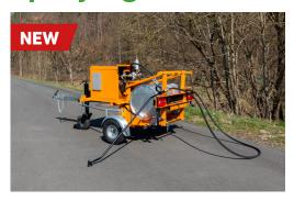
Bitumen emulsion spraying machine trailer for a 200 I drum forspraying pressure-sensitive adhesive and polymer-modified bitumen emulsions.
