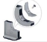
**Base**The die-cast moulded part is used as a practical connection between the cantilever rail and support profile. The components are simply inserted into the mounting sleeves and locked with just one screw. The support height inside the sleeve can be varied by up to 30 mm. The non-slip protective cap on the underside of the base prevents damage to the seal.
