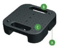
**Counterweights**The counterweights offer the following advantages: – No sharp corners or edges (A) – No damage to roof seal – Tamper-proof screw fitting – Easy to transport with carrying handles (B) – Space-saving storage and transport thanks to flat shape (C) – Weight (25 kg) complies with standard
