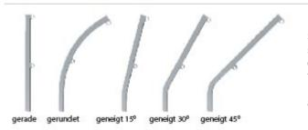
**Supports**Barrial® Self-supporting has 5 different support shapes to choose from. The system blends discreetly into the building architecture and the look of the facade thanks to the curve (1000 mm radius) or pitch (15°, 30° or 45°). The inward pitch provides an additional safety gap to the roof edge.
