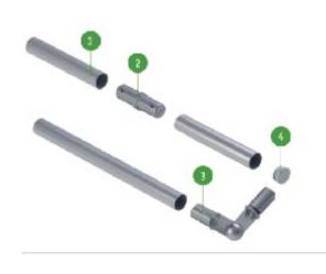
**Railing profiles and accessories** The aluminium system components are light and practical to handle. Hand and knee rails are discreet and evenly proportioned. The butt connectors, corner connectors and wall clamps with spreading technology ensure a secure hold and can be fitted with one tool to save time. The system adapts easily to a wide rang of building geometries with its variable angle corner connectors. 1) Railing profile 2) Butt connector 3) Variable angle corner connector 4) End cap
