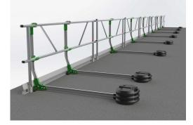
Temporary guardrail made of strong aluminium profiles with a max. support gap of 2.8 m, can also be used with edging board on flat roofs without parapet, up to max. 10° pitch
