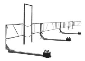
Temporary guardrail made of strong aluminium profiles with a max. support gap of 5.8 m for roof surfaces with up to  $10^{\circ}$  pitch or with accessories for gabled roofs up to  $18^{\circ}$
